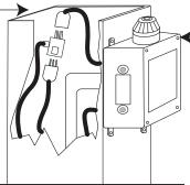
All electrical wiring in gas-tight and water proof UL Listed Alarm System (Enclosure is UL type 4X)
