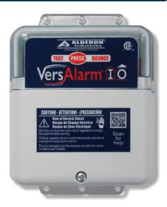
The VersAlarm™ I/O 1-Zone Alarm is an indoor and outdoor rated alarm panel, powered by 120VAC or 230VAC with conduit connections (required). When powered, the green LED will illuminate inside the top cover of the enclosure to indicate the unit is powered on. This alarm can be used for a wide variety of applications, including but not limited to: septic tanks, sump pits, holding tanks, pump chambers, and water tanks. Available in 120VAC or 230VAC models.
