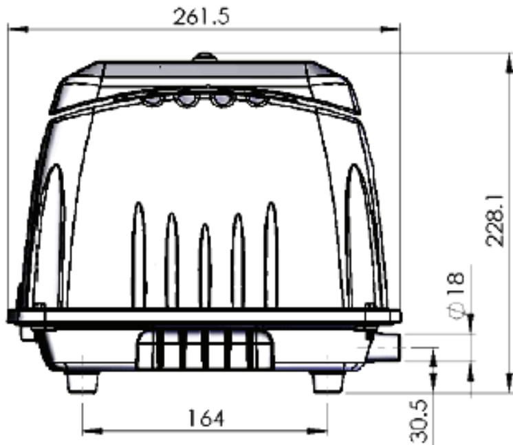
Dimensions measured in mm
