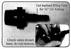
1. <sup>3</sup>/<sub>4</sub>" MPT barbed check valve is designed to be used with <sup>1</sup>/<sub>2</sub>" and <sup>3</sup>/<sub>8</sub>" I.D. tubing. Remove end of barb if installing <sup>1</sup>/<sub>2</sub>" I.D. tubing.
