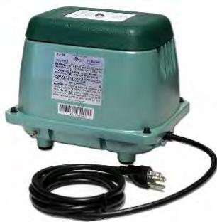
The Air Pump has an attached cord and will simply plug into any existing 115 V receptacle. When 115 volt electrical connections have been made turn on power. The air pump does not have an On/Off switch and should run as soon as power is applied.
