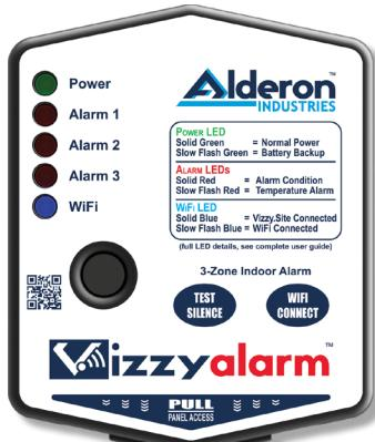
NOTE: If zone-1 is in an alarm condition and the buzzer is silenced, and then zone-2 and/or zone-3 goes into an alarm condition, the buzzer will reactivate until the test/ silence pushbutton is pressed to acknowledge that a new alarm condition has occurred.
