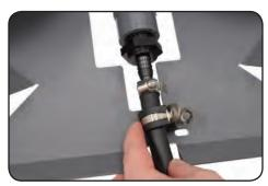
6. Fit padded hose clamp over tubing. (Use 17.5mm clamp for <sup>3</sup>/<sub>8</sub>" tubing or 25.5mm clamp for <sup>1</sup>/<sub>2</sub>" and <sup>5</sup>/<sub>8</sub>" tubing)
