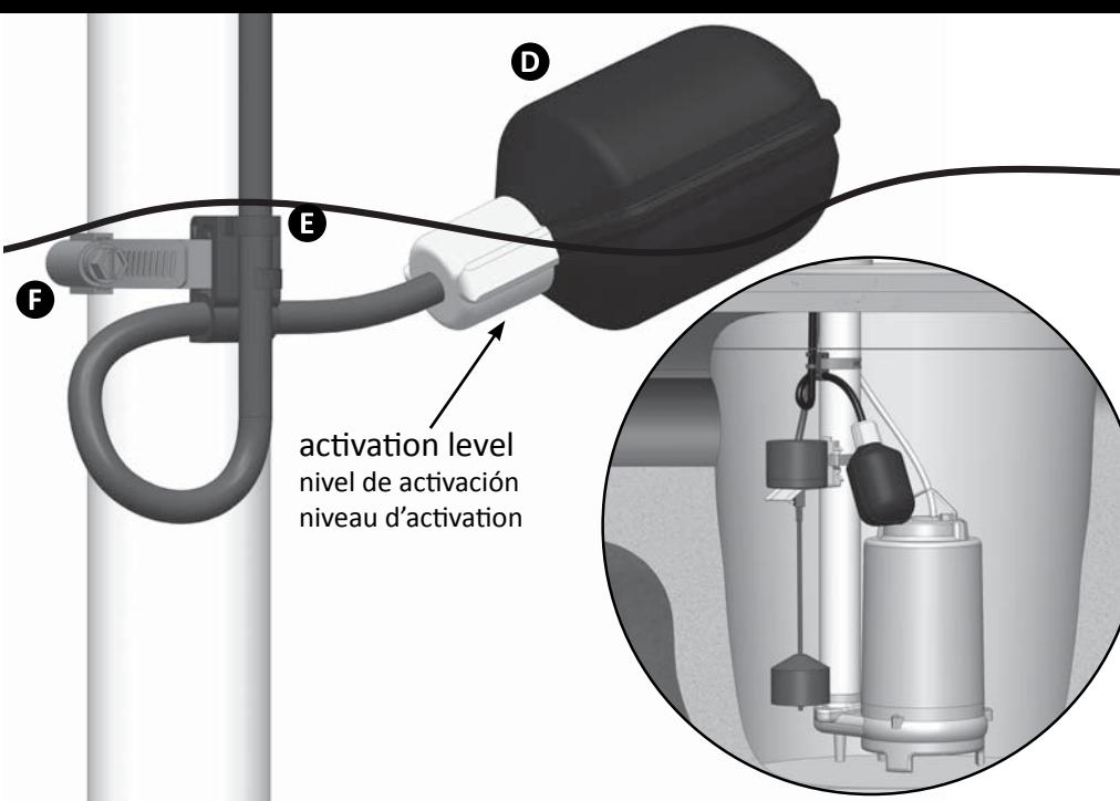
**5** Restore power and check alarm operation after installation.
