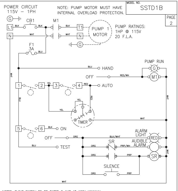
NOTES: FLOAT SWITCH TO BE RATED 2 AMP AT 120V MINIMUM. MAIN PANEL DISCONNECT MUST BE PROVIDED BY INSTALLER. DASHED LINES INDICATE ITEMS NOT CONTAINED IN THE PANEL. FIELD WIRING MUST BE A MINIMUM OF 60°C COPPER WIRE. TO PRESERVE ENVIRONMENTAL RATING OF PANEL, USE FITTINGS AND HUBS WITH SAME ENVIRONMENTAL RATING AS ENCLOSURE
