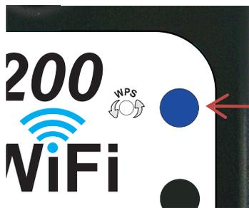
The blue network status light will illuminate steadily when the CS1200 WiFi Alarm is successfully connected to the wireless network.
