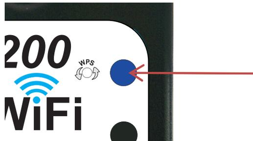
The blue network status light will illuminate steadily when the CS1200 WiFi Alarm is successfully connected to the wireless network.
