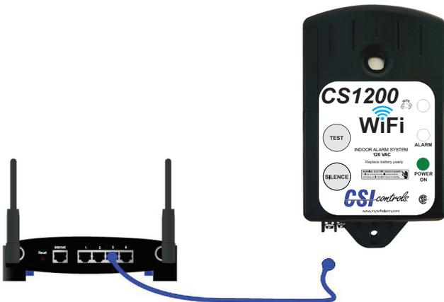
1. Connect an Ethernet cable (not supplied) from the CS1200 WiFi Alarm Ethernet port to a unused network router LAN port.
