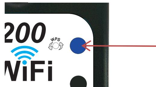
The blue network status light will illuminate steadily when the CS1200 WiFi Alarm is successfully connected to the Ethernet network.
